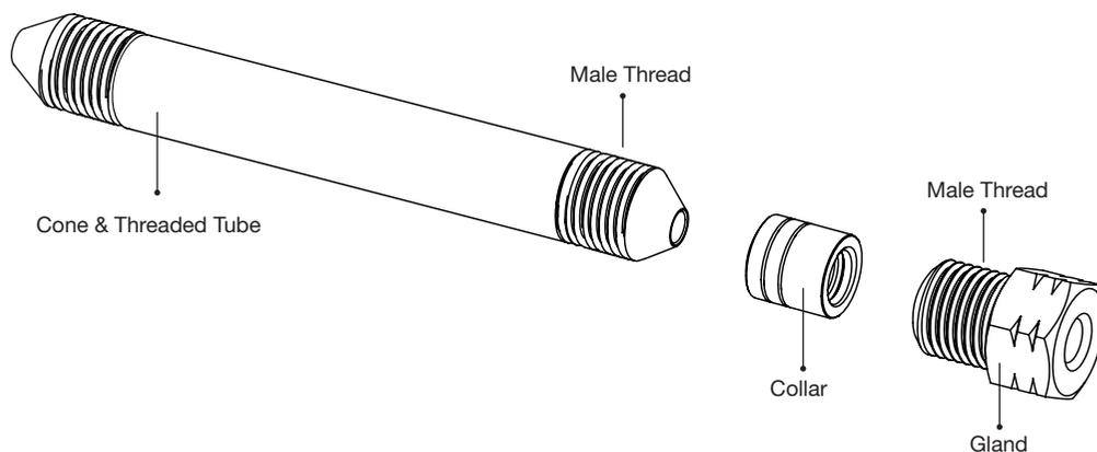
1. Lubricate all male threads with any anti-seize lubricant.
