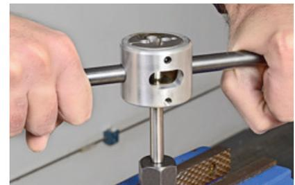
Place the palm of your hand firmly against the center of the threading tool and rotate your wrist counterclockwise. This will help "start" the die onto the tube. After you feel the die start onto the tubing, continue to rotate the threading tool using the handles. Remove the threading tool and clean off cutting fluid and chips.
