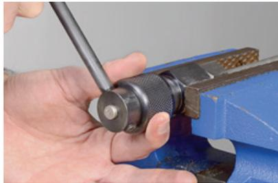
Rotate handle of cutting tool clockwise fairly rapidly with one hand while slowly rotating the knurled cap clockwise with the other hand in order to continuously feed the cutter into the tubing. Do not overly force the cutter against the tubing as it will bind. (You will quickly develop the proper feel).
