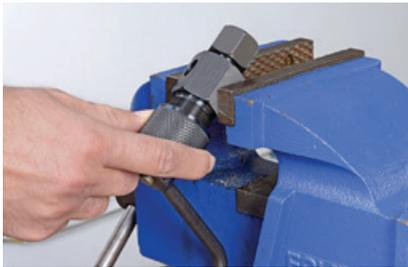
Secure the coning tool body in suitable in the vise. Angle position is preferred to have better access to the collet nut and knurled cap. Rotate the knurled cap clockwise into the tool as far as it will go.
