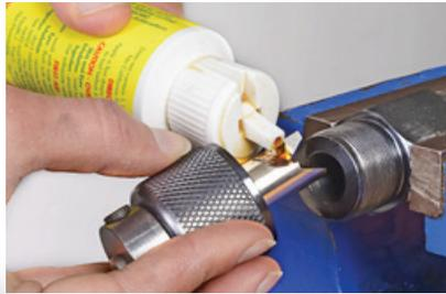
Turn knurled cap counterclockwise to remove cap and cutter from tool. Apply a very liberal amount of cutting fluid to the end of the cutter. Screw cap and cutter back into the body until the cutter contacts the end of the tubing.
