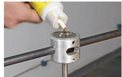
Apply a liberal amount of cutting fluid to the end of the tubing. Place the threading tool (guide bushing side first) onto the tubing.
