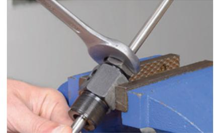
The coning tool (with the knurled cap and cutter removed) provides an ideal way to hold the tubing for the threading operation.
