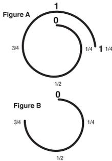
2. Tighten the nut. 1-1/4 turns of the nut is required for 1/4" (6 mm) and higher (See Figure A). 3/4 turns of the nut is required for 1/8" (See Figure B).
